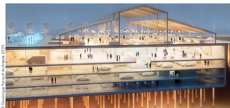
The term "deep square" refers to a public square with integrated facilities below ground which are used either to serve a multipurpose market hall or to free up public areas on the surface and leave them as unobstructed as possible.
